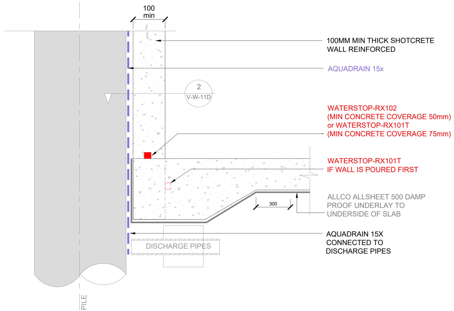
1 SHOTCRETE WALL FOOTING DETAIL - "WET" WALL
