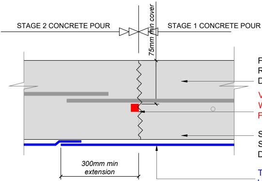
FLOOR SLAB REINFORCEMENT, REFER ENGINEERS DESIGN & DOCUMENTATION.
