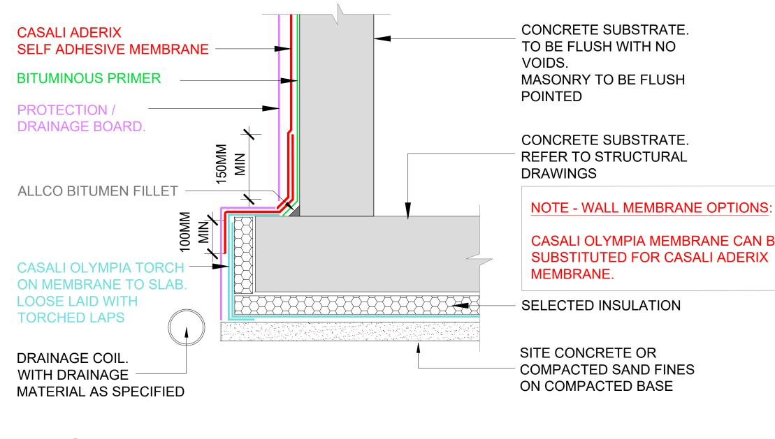
**RETAINING WALL / HEELED FOOTING JUNCTION TO INSULATED SLAB**
