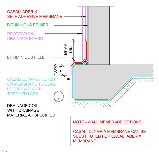
CONCRETE SUBSTRATE. TO BE FLUSH WITH NO VOIDS. MASONRY TO BE FLUSH **POINTED** CONCRETE SUBSTRATE. REFER TO STRUCTURAL **DRAWINGS** 100MM MIN ALLSHEET DPM OR SIMILAR. TAPED TERMINATION. SITE CONCRETE OR **COMPACTED SAND FINES** ON COMPACTED BASE
