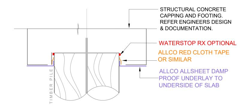
FOUNDATION DETAIL - TIMBER PILE / CAPPING BEAM DPM SCALE: NTS
