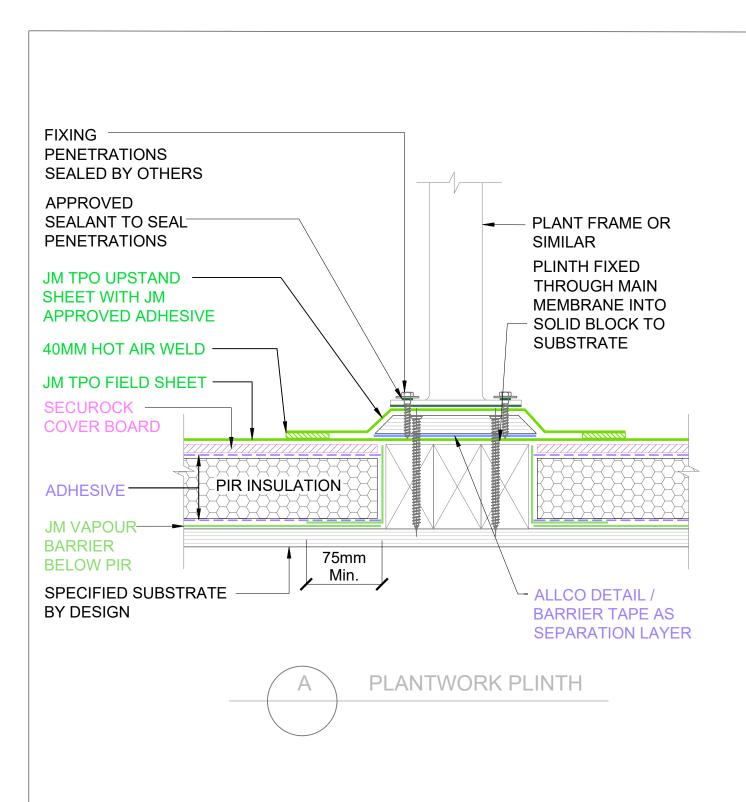
ALLCO ALLTHERM WARM ROOF - JM TPO -PLANTWORK FIXING PLINTH SCALE: NTS
