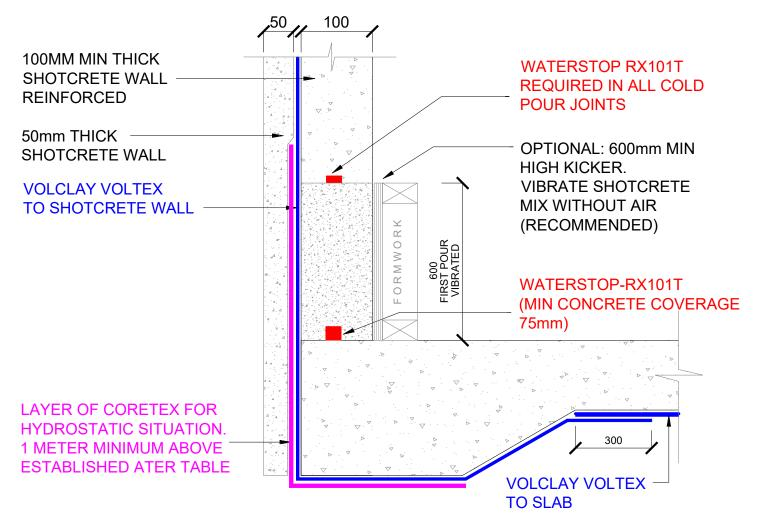
SHOTCRETE WALL FOOTING DETAIL (NON HYDROSTATIC) SCALE: NTS
