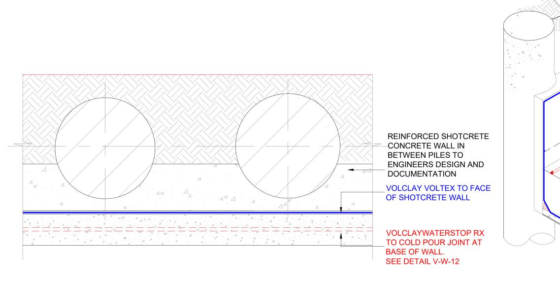
1 SHOTCRETE WALL - BASEMENT WALL SCALE: NTS
