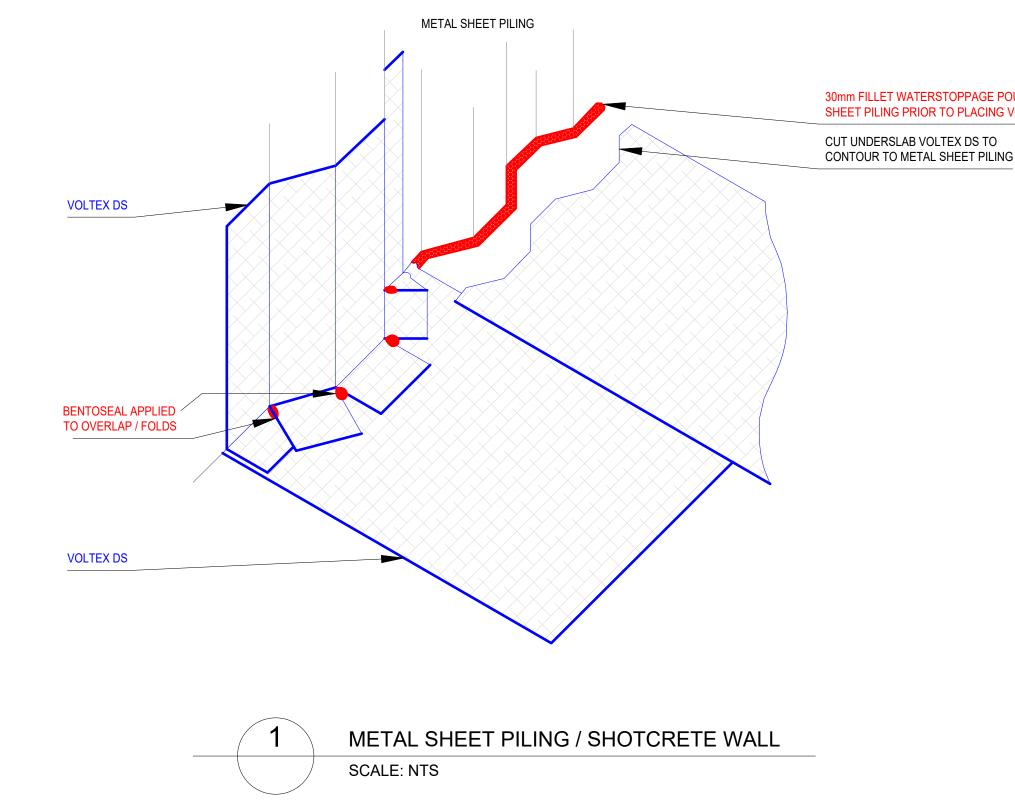
INSTALL VOLTEX WITH DARK GRAY (WOVEN) GEOTEXTILE AGAINST CONCRETE
