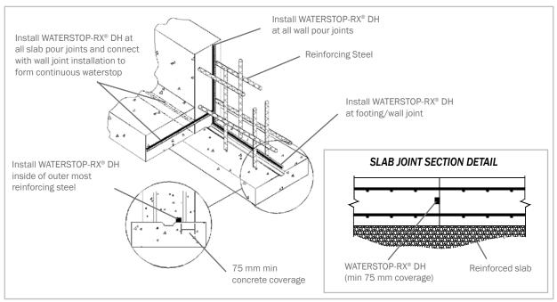
Typical WATERSTOP-RX® DH Foundation Detailing
