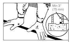
REMOVE RELEASE PAPER THEN PRESS FIRMLY AGAINST CETSEAL. MAINTAIN MIN. CONCRETE COVERAGE DEPTH
