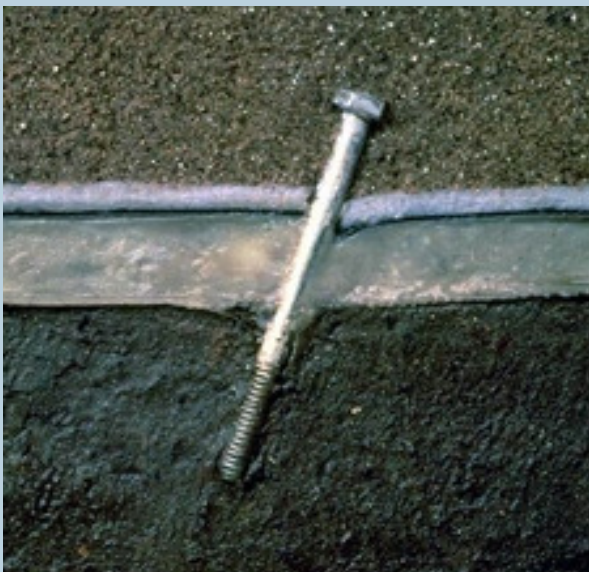
When hydrated, bentonite expands and conforms to penetrations and irregular surfaces, sealing small concrete cracks.
